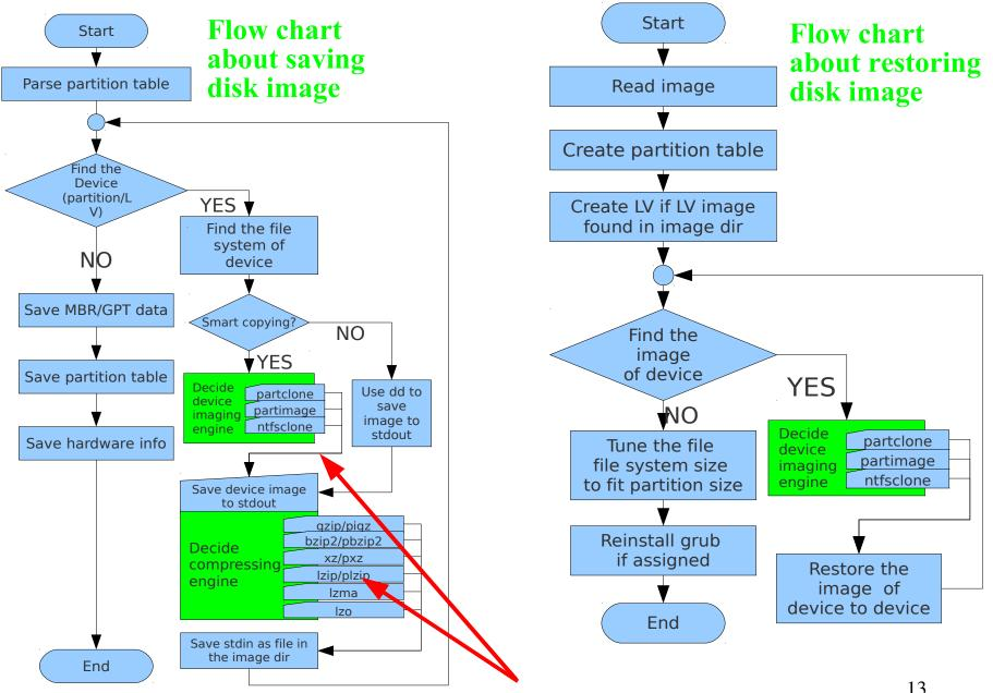
Imaging and compressing engines can be easily added
